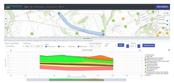
Sanitary sewer trenches are often in excess of 4 metres in depth and could potentially steal or divert groundwater away from local watercourses and fish habitat. Mitigation measures, such as trench plugs, may need to be incorporated into design concepts for this area. A detailed understanding of local hydrogeology/ groundwater features, potential development impacts, and mitigation measures need to be studied through a subwatershed study process.
