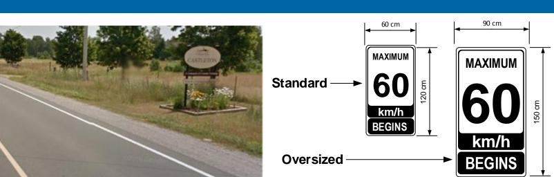
What It Is: Replacing standard sized signs with oversized signs and repositioning signs relative to each other and proposed pavement markings.
